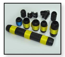
The rubber protectors are designed to protect the streamer from potential damage caused by bird collars, weights and digital modules when it is being wound onto the streamer reel. The protectors are molded to fit snugly over the collars, weights or modules and are fitted with Velcro™ straps to allow easy attachment to, or removal from, the streamer during retrieval or deployment.
