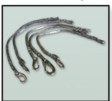
Seamap manufactures Safety Harnesses in various lengths and load ratings. While the breaking strength of the rope used in the harnesses is in excess of 2,500 Kg., the actual breaking strength of the entire assembly is dependent on the metal clip. The basic harness is supplied with a 60 mm hook and has a breaking strength of 450 Kg. while the strongest harness is fitted with a 90 mm clip and has a breaking strength of 1,800 Kg.
