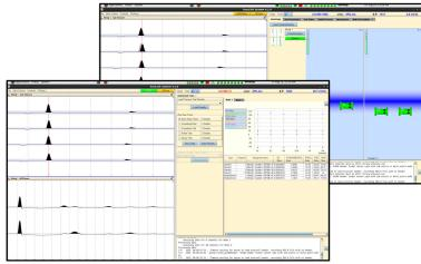
The unit provides onboard testing of individual Gun Fire and Sensor Module (GFSM) units and Termination Electronic Modules (TEMs). It's capable of determining whether they are working correctly either before, in the case of spares, or after being attached to the array once a fault has been reported.
