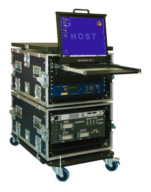
The GunLink Test Unit, sometimes referred to as an MRM (Mobile Rack Mounted) is a portable system designed for quick and easy onboard testing of individual GFSM and TEM.
