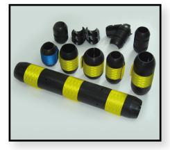
The rubber protectors are designed to protect the streamer from potential damage caused by bird collars, weights and digital modules when it is being wound onto the streamer reel. The protectors are molded to fit snugly over the collars, weights or modules and are fitted with Velcro<sup>™</sup> straps to allow easy attachment to, or removal from, the streamer during retrieval or deployment.
