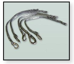
Seamap manufactures Safety Harnesses in various lengths and load ratings. While the breaking strength of the rope used in the harnesses is in excess of 2,500 Kg., the actual breaking strength of the entire assembly is dependent on the metal clip. The basic harness is supplied with a 60 mm hook and has a breaking strength of 450 Kg. while the strongest harness is fitted with a 90 mm clip and has a breaking strength of 1,800 Kg.
