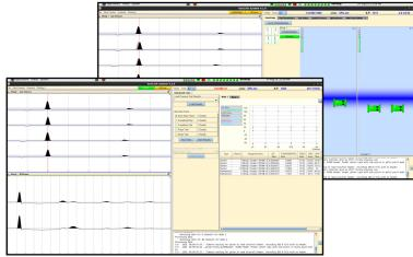
The unit provides onboard testing of individual Gun Fire and Sensor Module (GFSM) units and Termination Electronic Modules (TEMs). It's capable of determining whether they are working correctly either before, in the case of spares, or after being attached to the array once a fault has been reported.
