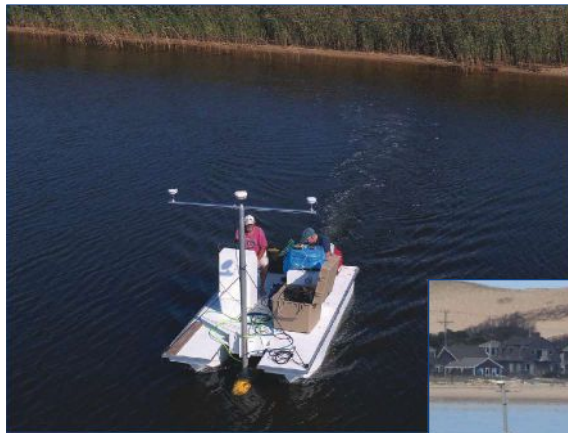
Shallow-draft survey vessels. Left: two-person, custom-built, pontoon boat (15-cm draft). Below: customized, 8.2-m Eastern. A bow-mount is preferred to reduce noise from hull and to maximize distance from engine. Both vessels pictured are using the EdgeTech 6205.
