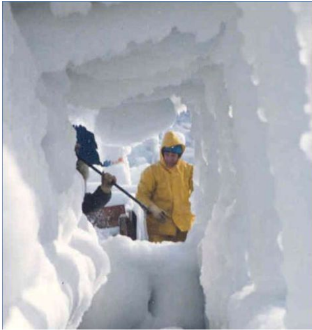
(Left) A dangerous coating of ice on the NOAA Ship Miller Freeman in the Bering Sea, Alaska. Such icing can affect a ship's stability and cause capsizing. (Photo Credit: NOAA Library Ship Collection, Courtesy of NOAA NMAO Pacific Marine Center) (Right) During a winter research cruise to the Labrador Sea in 1997, waves washing over the decks of the RV Knorr caused continual ice buildup. It took six to eight people the better part of a day to bang all the decks, bulkheads and bulwarks free of tons of ice. (Photo Credit: George Tupper, Woods Hole Oceanographic Institution)
