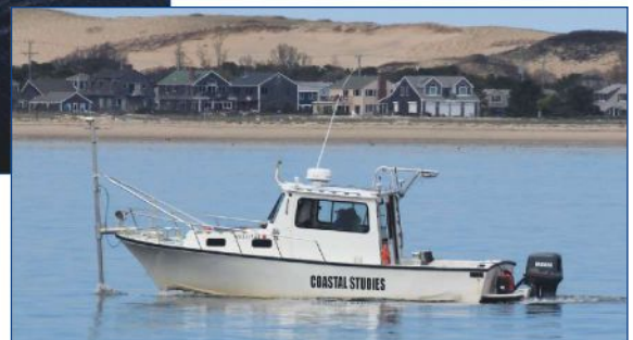
Shallow-draft survey vessels. Left: two-person, custom-built, pontoon boat (15-cm draft). Below: customized, 8.2-m Eastern. A bow-mount is preferred to reduce noise from hull and to maximize distance from engine. Both vessels pictured are using the EdgeTech 6205.
