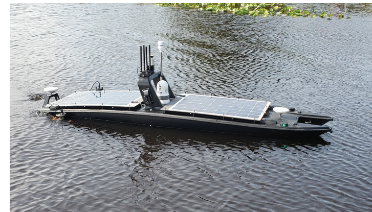
▲ Equipped with an environmental monitoring system and outfitted with solar panels, the MANTAS T12 is able to operate at sea uninterrupted for 30-day periods. (Photo credit: MARTAC)
