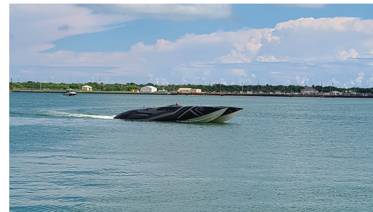
▲ MANTAS T38 DEVIL RAY, using a surveying speed up to 10-15kts, can stay underway for up to 8-10 days. (Photo credit: MARTAC)
