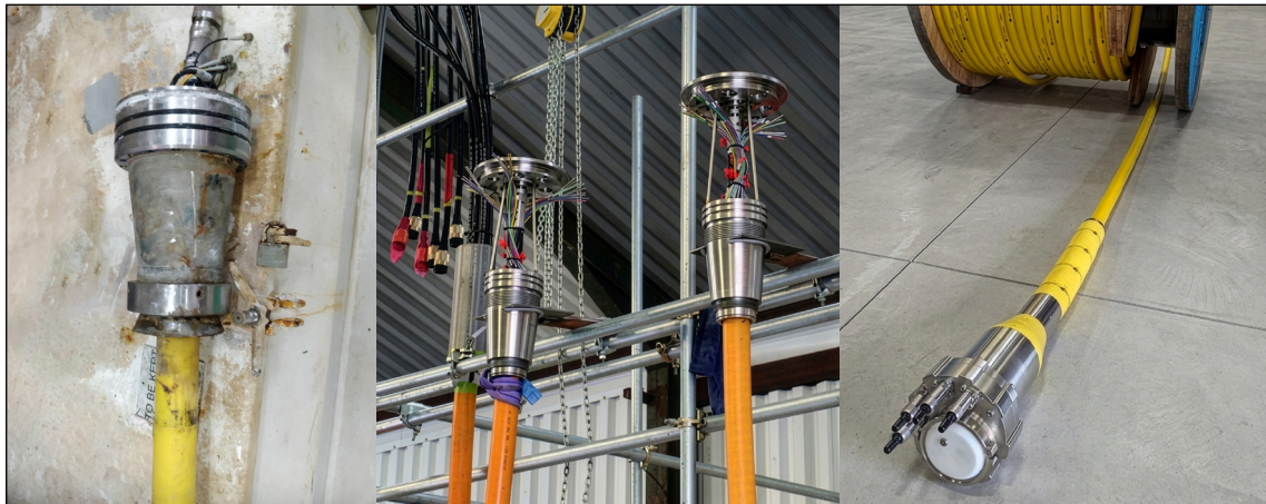
These images show the service stages from receiving (left) to repair and refurbishment (center) to finished product ready for deployment (right).
